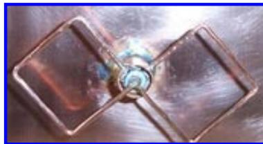
*solder the centre conductor to the element*
