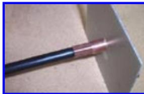
*the copper pipe crimped onto the coax*
