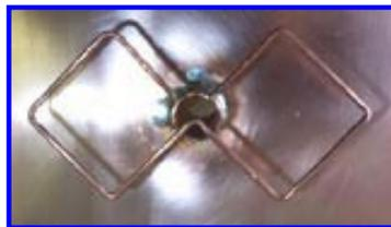
*the element soldered onto the copper pipe*
